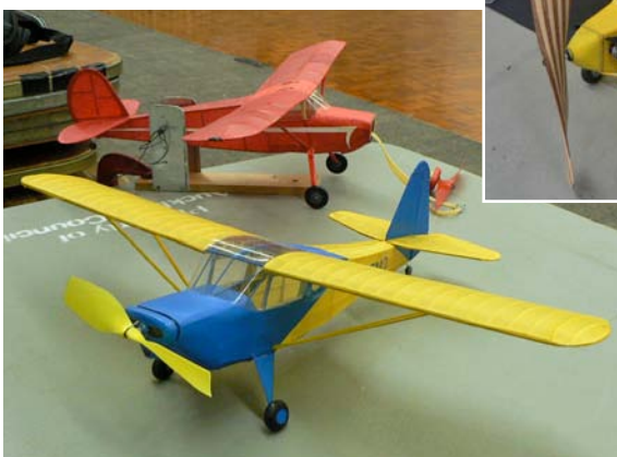
Upper: Keith Trillo's Peanut Scale Fike, showing winding tube and nicely built laminated propellor.
