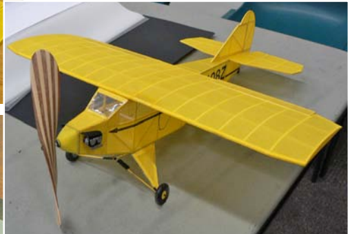
Upper: Keith Trillo's Peanut Scale Fike, showing winding tube and nicely built laminated propellor.
